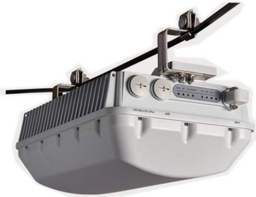
*Figure 1 - Ruckus T811-CM Wi-Fi access point can serve 512 users up to 1.7 Gbps. It is used by Google to provide free public Wi-Fi in Mountain View, CA. It consumes up to 93.7 watts of energy.*
